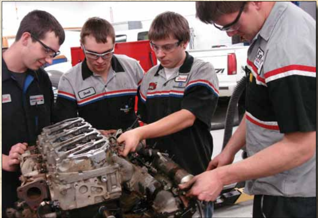
2012 ASEP graduates, from left, Mike Jones, Derek Langenberg, Dustin Smith, and Brady Prohaska perform engine disassembly procedures on a 6.6L Duramax Diesel engine.
