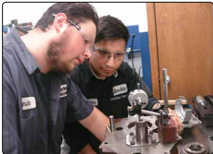
Dietrich Eggers, left, and Carlos Degante are checking the Countershaft Endplay on an NV 4500 manual transmission. Eggers is sponsored by Doug Meyer Chevrolet in Shenandoah, IA, and Degante is sponsored by Edwards Classic Chevrolet, Cadillac in Council Bluffs, IA.
